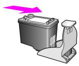
To remove the print cartridge from the print cartridge protector, press down and back on the top of the print cartridge protector to release the print cartridge, then slide the print cartridge out of the print cartridge protector.
