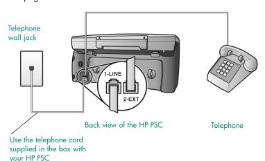
1 Using the phone cord supplied in the box with your HP PSC, connect one end to your telephone wall jack, then connect the other end to the port labeled "1-LINE" on the back of your HP PSC.
