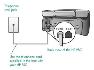
1 Using the phone cord supplied in the box with your HP PSC, connect one end to your telephone wall jack, then connect the other end to the port labeled "1-LINE" on the back of your HP PSC.
