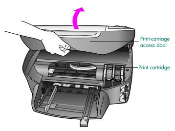
2 After the carriage stops moving and the ramp has lowered, lift the latch to up release the print cartridge.
