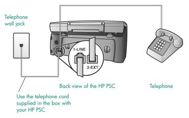
Using the phone cord supplied in the box with your HP PSC, connect one end to your telephone wall jack, then connect the other end to the port labeled "1-LINE" on the back of your HP PSC.
