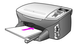
4 Slide the paper-width and paper-length guides inward until they stop at the edges of the paper. Make sure that the paper stack lies flat in the input tray and is stacked no higher than the paper-length guide.
