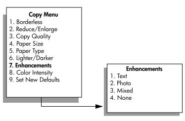
3 Press ▼ to highlight the Text enhancement setting, and then press OK.
