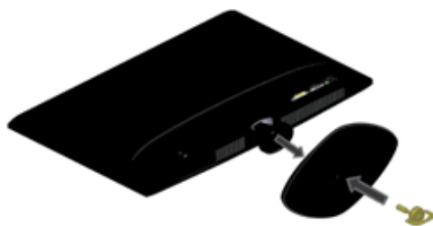
Figure 3-1 Installation de la base
