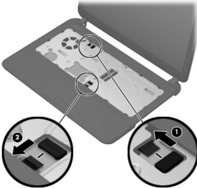
9. Lift the rear edge of the top cover **(1)** and swing it up and forward until it detaches from the computer.
