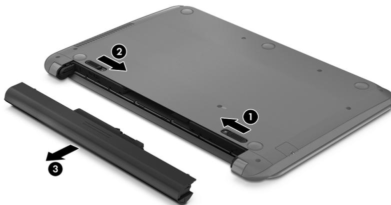
Reverse this procedure to install the battery.
