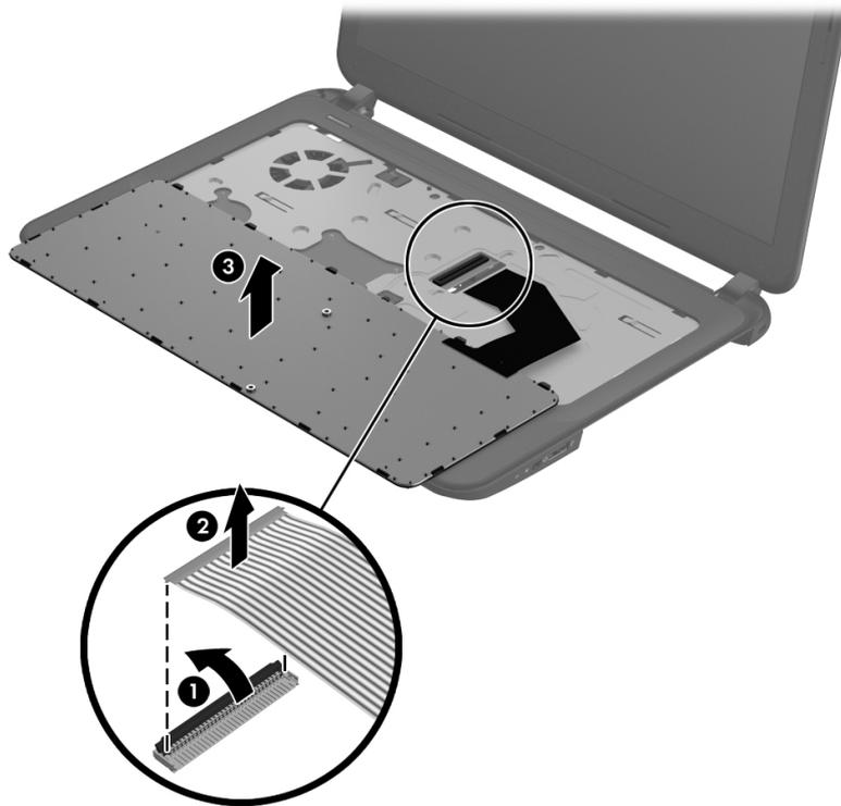
Reverse this procedure to install the keyboard.
